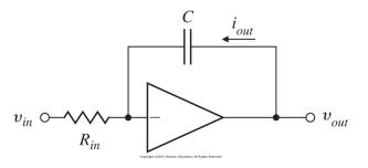
• (Example) Find a state-variable description and the transfer function of the system shown in the following figure whose differential equation is
