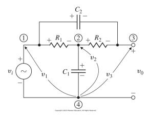
$$\frac{v_2 - v_i}{R_1} + \frac{v_2}{1/(C_1 s)} + \frac{v_2 - v_o}{R_2} = 0$$
