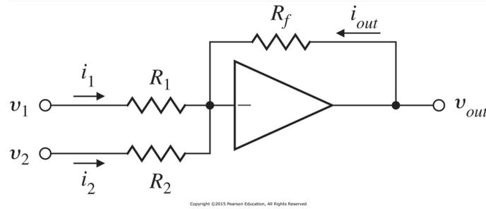
8. (Example 2.11, Op-Amp Summing Circuit) weighted sum of the input voltages with a sign change.
