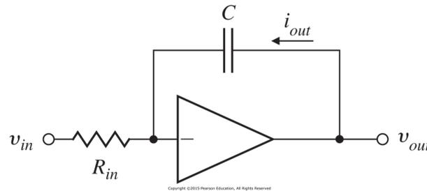
9. (Example 2.12, Op-Amp Integrator Circuit) integration of the input voltage with a sign change.
