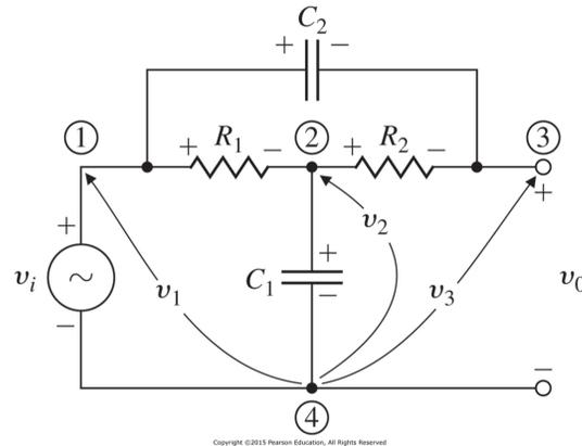
4. (Example 2.9, Bridged Tee Circuit) After assigning four node voltages, let us consider  $v_4 = 0$  as reference voltage, then we know  $v_1 = v_i$  and  $v_3 = v_o$  at nodes 1 and 3, respectively, and, at nodes 2 and 3, we have
