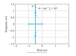
4. The dashed lines in Fig. 5.2 correspond to roots with a damping ratio  $\zeta = 0.5$  ( $\theta = \sin^{-1}\zeta = 30^{\circ}$ ). The crossing points denoted by dots can be calculated as follows:
