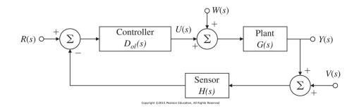
• (Example 4.3 System Type for a Servo with Tachometer Feedback) Consider Fig. 4.5 with  $G(s) = \frac{1}{s(\tau s+1)}$ ,  $D_c(s) = k_P$  and  $H(s) = 1 + k_t s$ . Determine the system type and relevant error constant with respect to the reference inputs when V = W = 0. The error TF is
